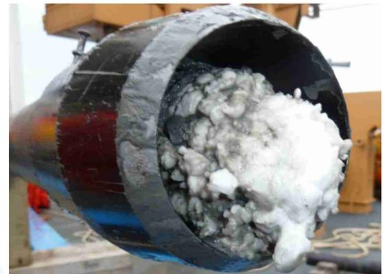
**Fig 1.** Especially when a pipeline is idle for a longer time at low temperatures, hydrate plugs can form, similar to the methane hydrate core shown in the picture.
