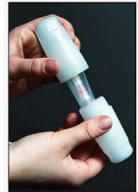
Fig 1. Encapsulation of the sample before packaging in an irradiation container. The container is positioned close to the nuclear reactor core via a pneumatic tube system.
